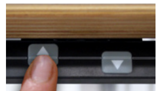
Motorverstellung M1 height adjustment by motor M1
